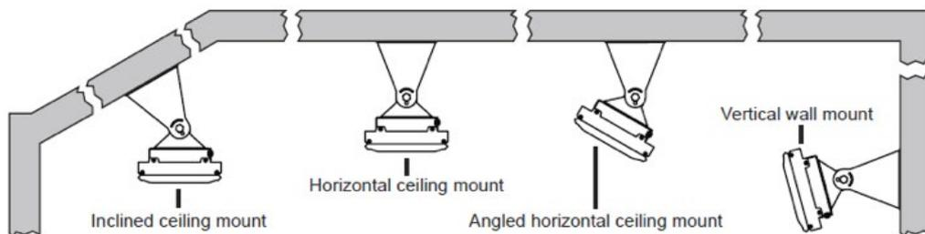
Mounting brackets are included with your purchase for easy installation in a variety of positions. Depending on the area and the available space, you may want to mount the heater on either the wall or the ceiling.
